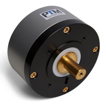
Radial piston motor Exclusively ferrite-free, non-magnetic materials For TESLA applications, MRI devices, medical technology, high-frequency applications Rotation speed 0-300 rpm reversible Four performance variants Noise level < 75 dB Oil and silicone-free Various drive shafts Housing aluminium anodised Compressed air supply 2-6 bar | 30-90 PSI Magnetic flux density <50pTpp\* Magnetic dipole moment <50nAm^\* (nano ampere meter square)
