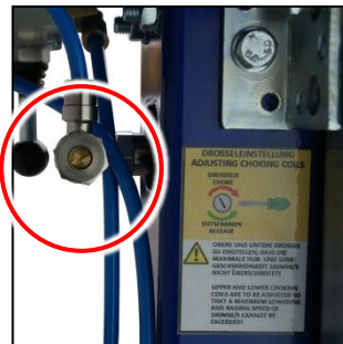
Lower throttle with lowering protection/ upper throttle internal orifice
