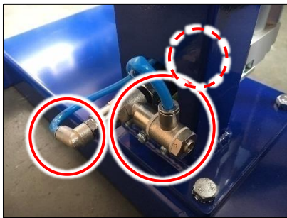
Lower throttle with lowering protection/ upper throttle internal orifice
